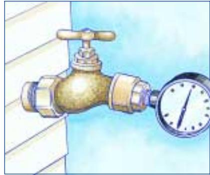
To check water pressure, attach a pressure gauge to the outside faucet nearest the water meter. A pressure gauge can be obtained from your local Hunter dealer.
