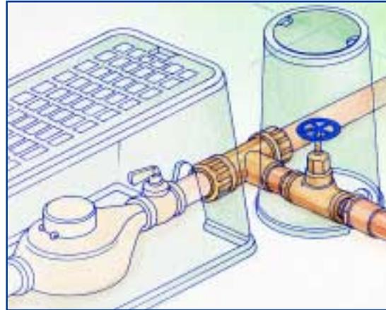
*P.O.C. Non-Freezing: Use a brass compression tee to connect your sprinkler system to the household water supply.*
