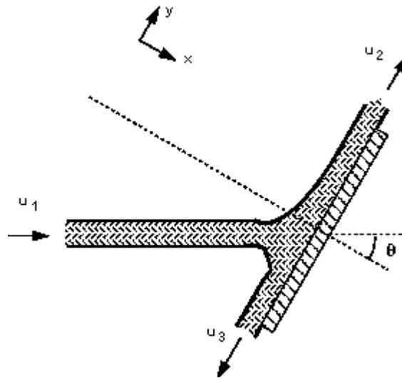
A jet hitting an inclined plane.
