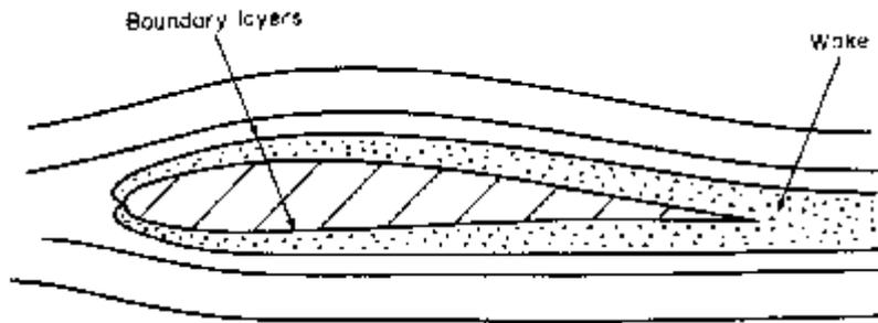
The velocity increases as air it flows over the wing. The pressure distribution is similar to that shown below so transverse lift force occurs.
