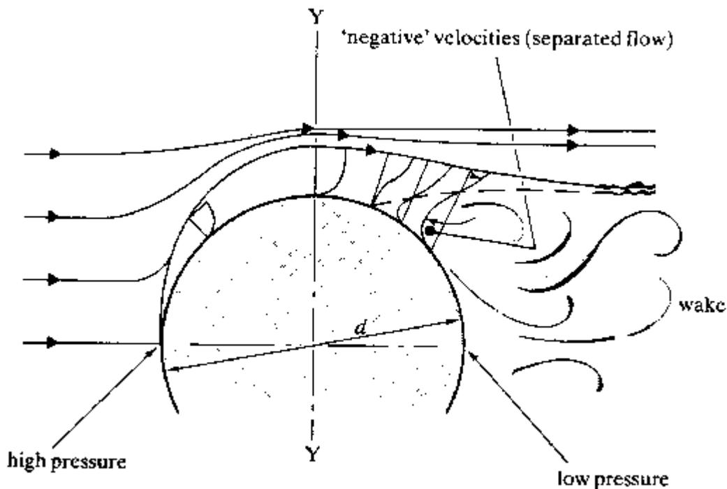
Looking at the figure above, the formation of the separation occurs as the fluid accelerates from the centre to get round the cylinder (it must accelerate as it has further to go than the surrounding fluid). It reaches a maximum at Y, where it also has also dropped in pressure. The adverse pressure gradient between here and the downstream side of the cylinder will cause the boundary layer separation if the flow is fast enough, ( $Re > 2$ .)
