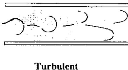
Actually both would happen - but for different flow rates. The top occurs when the fluid is flowing fast and the lower when it is flowing slowly.
