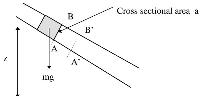
An element of fluid, as that in the figure above, has potential energy due to its height  $z$  above a datum and kinetic energy due to its velocity  $u$ . If the element has weight  $mg$  then
