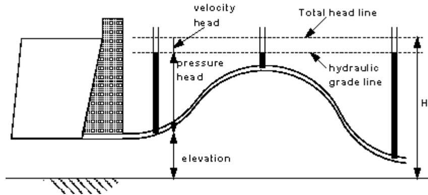
Piezometer levels when fluid is flowing
