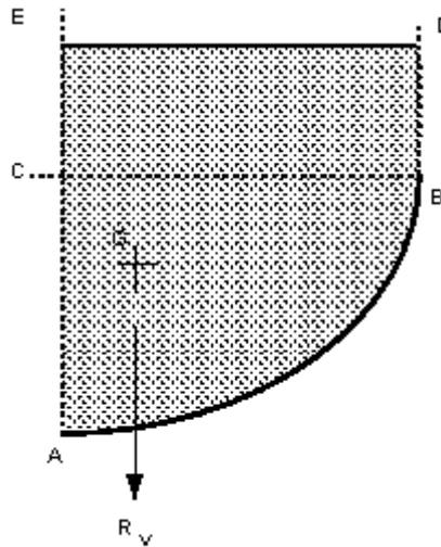
There are no shear force on the vertical edges, so the vertical component can only be due to the weight of the fluid. So we can say
