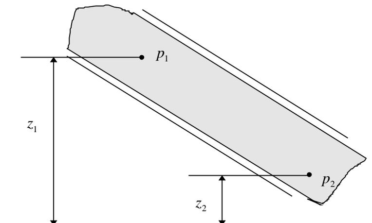
The pipe is filled with stationary fluid of density  $\rho$  has pressures  $p_1$  and  $p_2$  at levels  $z_1$  and  $z_2$  respectively. What is the pressure difference in terms of these levels?
