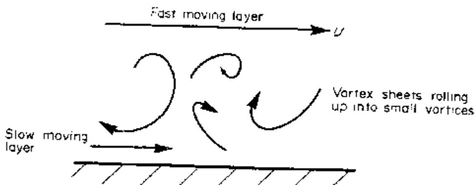
This causes the fluid motion to rapidly become turbulent. Fluid from the fast moving region moves to the slower zone transferring momentum and thus maintaining the fluid by the wall in motion. Conversely,
