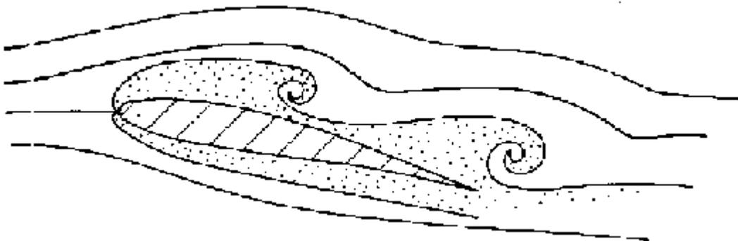
When stalling occurs, all, or most, of the 'suction' pressure is lost, and the plane will suddenly drop from the sky! The only solution to this is to put the plane into a dive to regain the boundary layer. A transverse lift force is then exerted on the wing which gives the pilot some control and allows the plane to be pulled out of the dive.
