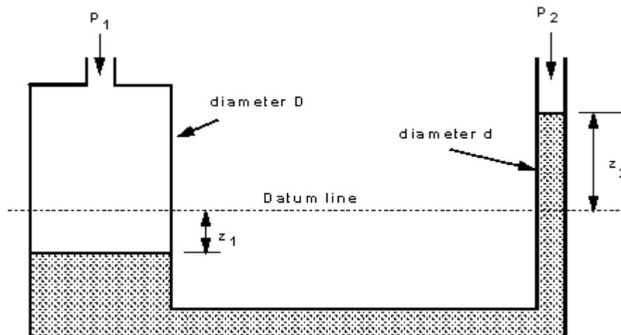
Assume the manometer is arranged as above to measure the pressure difference of a gas of (negligible density) and that pressure difference is  $p_1 - p_2$ . If the datum line indicates the level of the manometric fluid when the pressure difference is zero and the height differences when pressure is applied is as shown, the volume of liquid transferred from the left side to the right =  $z_2 \times (\pi d^2 / 4)$
