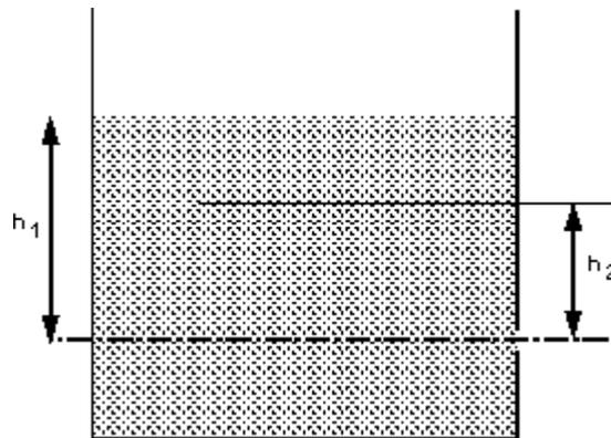
Tank emptying from level  $h_1$  to  $h_2$ .
